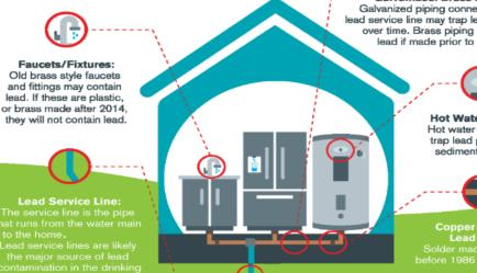
Galvanized/Brass Pipes: Galvanized piping connected to a lead service line may trap lead particles over time. Brass piping contains lead if made prior to 2014.
