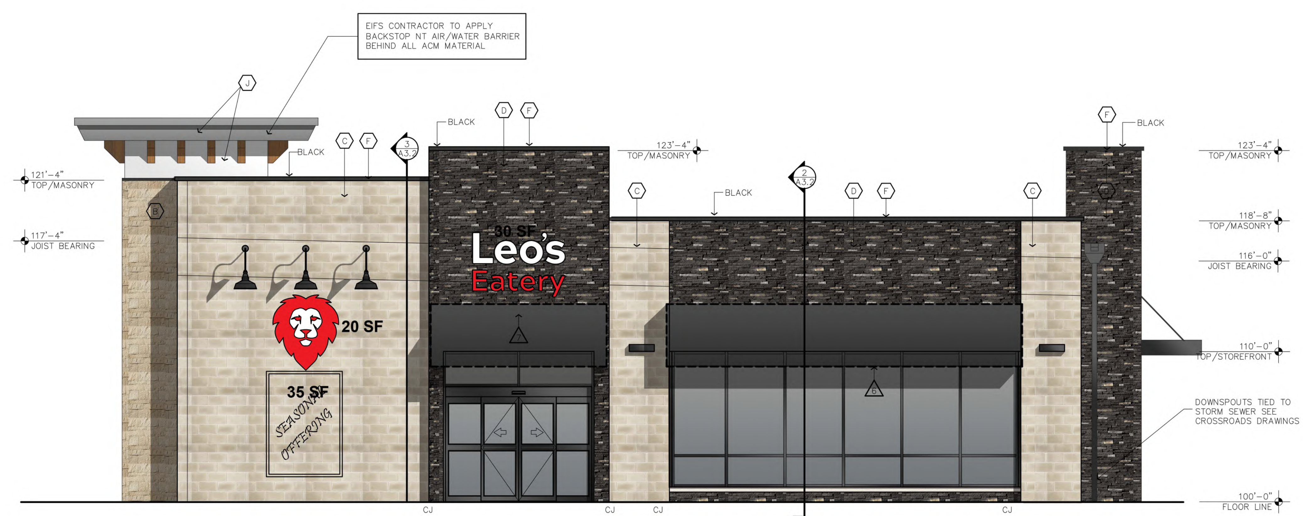
RIGHT SIDE ELEVATION SCALE: 1/4"=1'-0" NORTH SIDE OF BUILDING TOTAL SIGNAGE AREA = 85 sft
